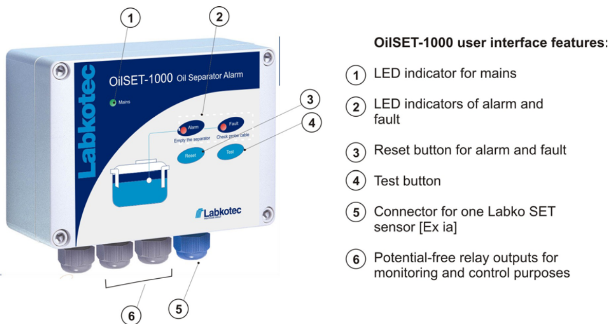
Figure 2. OilSET-1000 control unit - features
