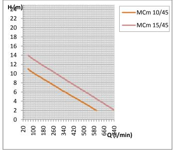
These pumps are suitable for rainwater with small pollution, such as mud in emptying building sellers, water after a water treatment plant, ...
